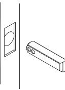
INSERT BOLT INTO CARRIER NOTE: HOLES INDICATE FOR 2 3/4 OR 2 3/8 DOOR WIDTH SEE STEP 2
