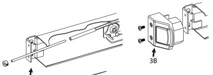
3C: SET EXIT DEVICE TO THE DOGGED POSITION. TO ADJUST THE ACTUATING ROD, PUSH ROD THROUGH THE HOLE IN END CAP UNTIL IT CONTACTS THE BACKSIDE OF THE BUTTON, SLIDE LOCKING COLLAR BACK UNTIL IT CONTACTS THE TUBE AND TIGHTEN FIRMLY.
