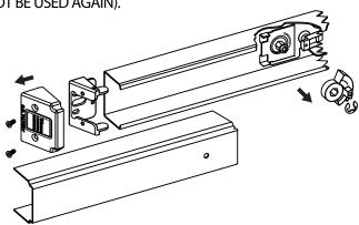
INSTALL CAM ONTO HEX POST, ALIGN DETENT BALL WITH CENTER NOTCH (UNDOGGED, FIG 2.1). **INSTALL RETAINING RING ON** TOP OF THE CAM INTO GROOVE ON HEX SHAFT, (CONVEX SIDE UP/FIG. 2.2).
