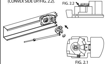
REINSTALL DORMA MOUNTING BRACKET, INSTALL TRIMCO END CAP BY USING PROVIDED PHILLIPS 8-32 MACHINE SCREWS.
