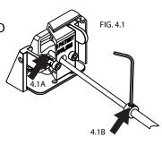
WITH END CAP AND MOUNTING BRACKET REMOVED SLIDE IN COVER.
