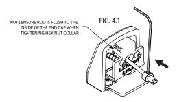
REPLACE LDH100-VD END CAP BY USING THE PROVIDED HEX L-WRENCH TO LIFT AND GUIDE THE SHAFT INTO THE HOLE LEADING TO THE BUTTON. REPLACE WITH PHILLIPS #10-16 X 3/8"T-CUT SCREWS.
