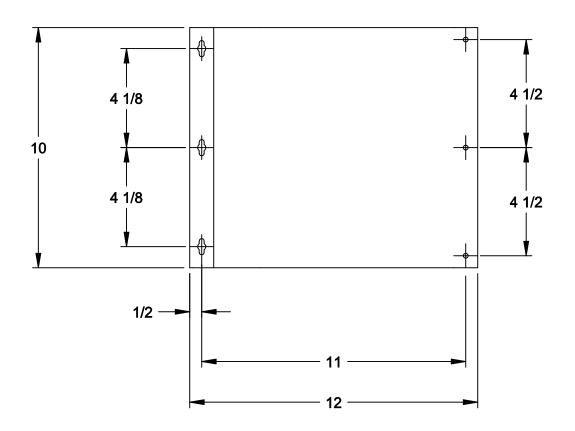
SUPPLIED WITH: SIX (6) #6 X 5/8" TRUSS HEAD, PHILLIPS DRIVE WOOD MOUNTING SCREWS.
