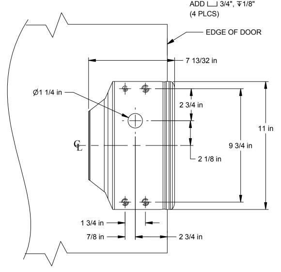
FOR SINGLE DOORS ONLY (CONTACT FACTORY FOR DOUBLE DOOR INSTALLATION) DO NOT USE THIS TEMPLATE IF MATING TO RIM, EXIT, OR PANIC DEVICES.
