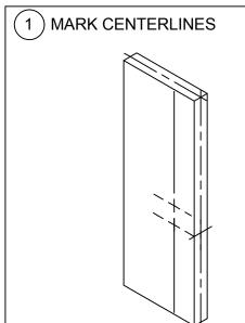
Mark the horizontal centerline of the lock Position the applicable Template on both sides of the door and on door's on the edge and the sides of door edge.
