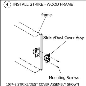
Prep door frame per applicable Template, Sheet 3, and install strike/dust cover assy.
