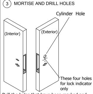
Drill the holes that have been marked and mortise door - Reference applicable Templates, Sheets 1 &2, for hole dia/depth and mortise prep specifications.
