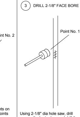
perpendicular to door and drill through.
