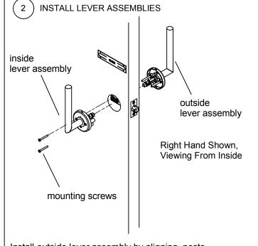
Install outside lever assembly by aligning posts with corresponding posts of inside lever assembly. Attach inside knob assembly by fastening two (2) screws.
