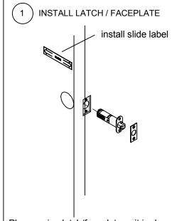
Place spring latch/faceplate unit in door making sure bolt bevel faces direction of door closing. Install latch and loosley fasten with two (2) wood screws. Verify that the outer face of the faceplate is flush to door.
