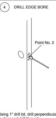
Using 1" drill bit, drill perpendicular to door and drill through.
