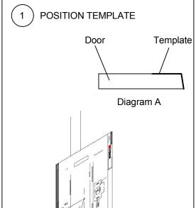
Cut template where indicated. Fold enclosed latch template on dotted line and locate on door at desired height. If door is beveled (See Diagram A). Place folded edge on shorter side of bevel as shown above. Tape latch template in place.
