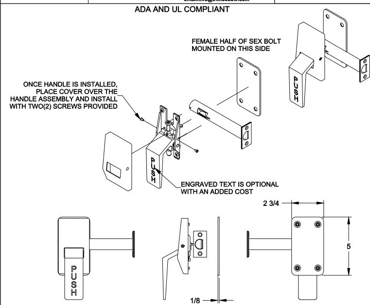
SUPPLIED WITH FOUR (4) 1/4-20 SEX BOLTS FOR MOUNTING HANDLE AND PLATE - DOOR PREP FOR SEX BOLT - DRILL Ø5/16 HOLES. ALSO SUPPPLIED WITH TWO (2) #8 X 3/4 COMBO SCREWS FOR MOUNTING THE LATCHBOLT.
