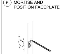
Slide latch into mortise. Check that screw mounting points are centered before tracing the outline of the faceplate. Chisel for faceplate to a depth of 5/32".
