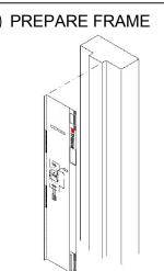
Tape strike template at matching centerline to latch template. Mark points. Position strike over frame and trace outline. Using 1"drill bit, Drill latch depth to 1-1/8" deep. Chisel out strike plate to a depth of 7/64".
