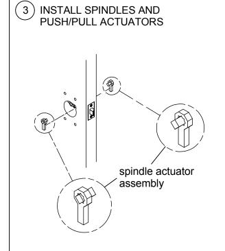
Install spindles and actuators as required by function. (Not provided for fixed or rigid handles)
