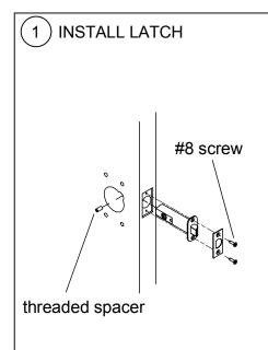
Place latch bolt unit in door. Making sure bolt bevel faces direction of door closing. Attach front with 2 (two) #8 screws. Install threaded spacer into latch.
