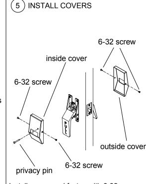
Install covers and fasten with 6-32 screws. Insert privacy pin through inside cover and thread into place.
