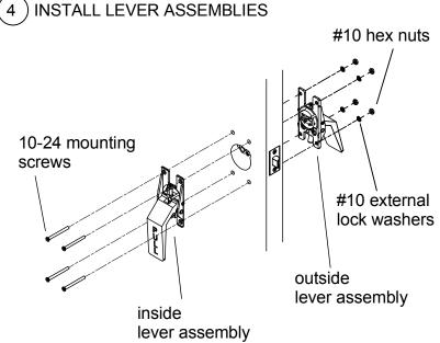
Install lever assemblies by aligning screws of inside lever assembly with corresponding holes in door. Verify handing for each assembly before mounting. Align lever assemblies and fasten with four (4) 10-24 mounting screws, four (4) external lock washers and four (4) hex nuts.
