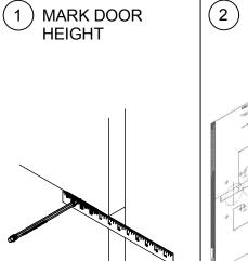
Draw a horizontal line on both sides of the door to indicate desired height of lever. (45" above floor suggested unless otherwise directed)
