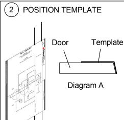
Fold (or cut if desired) enclosed latch template on dotted line. Align the line just marked on the door with the latch centerline which is on the latch/lever assy template. Tape template to door.
