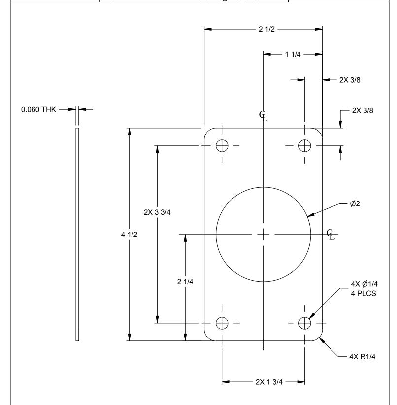
REVISION RECORD: 09/01/15 REVISION: REDRAWN IN CAD, 4X R1/4 WAS 4X CHAMFER, SUPERCEDES 05/23/02 DWG #11403, DLS 4X Ø1/4 4 PLCS WAS: 4X Ø3/8 4 PLCS, SGH/JG, 09/08/15
