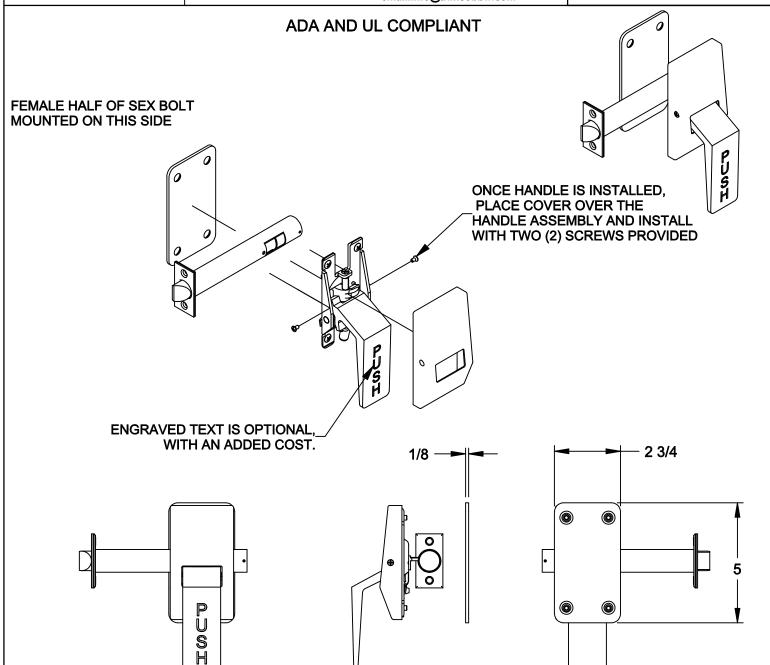
SUPPLIED WITH FOUR (4) 1/4-20 SEX BOLTS FOR MOUTNING HANDLE AND PLATE -. DOOR PREP FOR SEX BOLT - DRILL  $\emptyset$ 5/16 HOLES. ALSO SUPPLIED WITH TWO (2) #8 X 3/4 COMBO SCREWS FOR MOUNTING THE LATCHBOLT.
