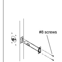
Place latch bolt unit in door, Making sure bolt bevel faces direction of door closing. Attach front with 2 (two) #8 screws.
