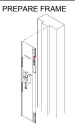
Tape strike template at matching centerline to latch template. Mark hole centers. Position strike over frame and trace outline. Chisel to a depth of 3/32" to accomodate strike plate.
