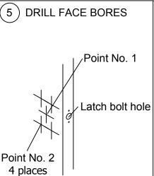
Using a 2 1/8" dia hole saw drill through at point 1. Using 5/16" dia drill bit drill through at point 2 (4 places). Using 1" dia to a depth of 4 3/8" for 2 3/4" backset, or 6 5/8" for 5" backset. 6 **MORTISE AND POSITION FACEPLATE**
