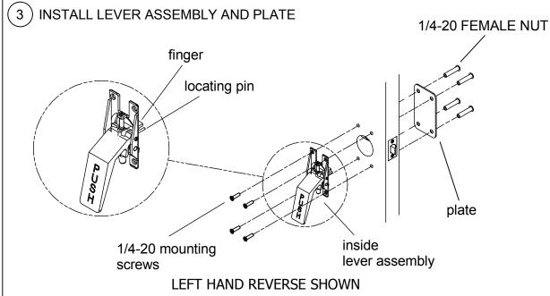
Install lever assembly by aligning the mounting holes of the inside lever assembly with the corresponding holes in the door, by inserting the finger into the latch cutout, and inserting the locating pin in the corresponding hole in the latch. Verify handing for each assembly before mounting. Align lever assembly and plate and fasten with four (4) 1/4-20 mounting screws, and four (4) 1/4-20 female nuts.
