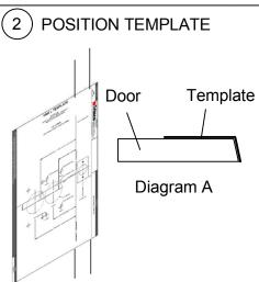
Fold (or cut if desired) enclosed latch template on dotted line. Align the line just marked on the door with the latch centerline which is on the latch/lever assy template. Tape template to door.
