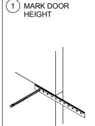
Draw a horizontal line on both sides of the door to indicate desired height of lever, (45" above floor suggested unless otherwise directed).
