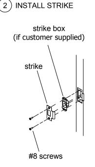
(3651 "B" strike shown) Install strike and strike box (if customer supplied) using two (2) #8 screws.
