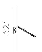
Slide latch into mortise. Check that screw mounting points are centered before tracing the outline of the faceplate. Chisel for faceplate to a depth of 5/32".
