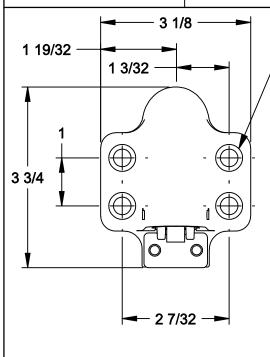
SUPPLIED WITH: FOUR (4) EACH OF THE FOLLOWING #14X1-1/2 FH, PH, SMS, 1/4-20X1-1/4 FH, PH, UC, MS AND #14X1-1/2 PLASTIC BANTAM PLUG
