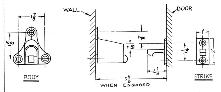
ROLLER AND STRIKE SHOULD BE IN COMPLETE CENTER ALIGNMENT CAN BE INSTALLED ON TOP RAIL , BOTTOM RAIL OR ANY INTERMEDIATE POSITION ON THE DOOR.
