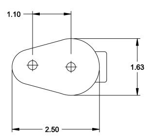
SUPPLIED WITH ONE (1) 5/16-18X1 LEAD ANCHOR, ONE (1) 1/4-20x7/8 LEAD ANCHOR, ONE (1) 1/4-20 X 1-1/4" FLAT HEAD, PHILLIPS DRIVE MACHINE SCREW, ONE (1) #14 X1-1/2 FLAT HEAD, PHILLIPS DRIVE SHEET METAL SCREW, ONE (1) 5/16-18 X 2 HANGER BOLT, ONE (1) 5/16 X 2 THREADED STUD AND ONE (1) #14-16X1-1/4 PLASTIC BANTUM
