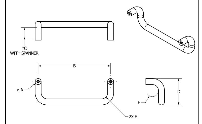
SUPPLIED WITH TWO 3/8-16 LH AND 3/8-16 RH THREADED STUDS, TWO SPANNER TURNING WASHERS AND TWO R5 RIV-NUTS, 5/16-18 RH FOR HOLLOW METAL DOORS
