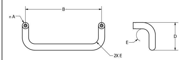
SUPPLIED WITH TWO 5/16-18 X 2-1/4" SHOULDER BOLTS AND FOUR 1/4-28 X 5/16" SET SCREWS
