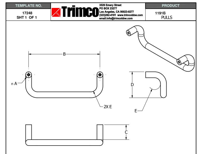
SUPPLIED WITH TWO 5/16-18 X 2.5 FLAT HEAD, PHILIPS DRIVE MACHINE SCREWS AND TWO 5/16 FINISH WASHERS.
