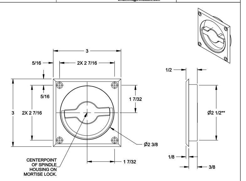
SUPPLIED WITH FOUR (4) #6 X 1 OVAL HEAD, PHILLIPS DRIVE SHEET METAL MOUNTING SCREWS AND FOUR (4) #6 X 5/8 OVAL HEAD, PHILLIPS DRIVE SHEET METAL MOUNTING SCREWS
