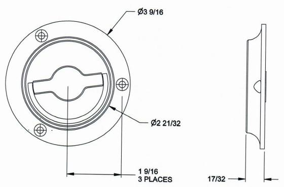
SUPPLIED WITH THREE (3) #8 X 1 OVAL HEAD, PHILLIPS DRIVE SHEET METAL MOUNTING SCREWS AND THREE (3) #8 X 5/8 OVAL HEAD, PHILLIPS DRIVE SHEET METAL MOUNTING SCREWS
