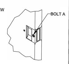
3. BOLT "A" ADJUSTS WIDTH OF PULL PAIR, AUTOMATICALLY ALIGNS PULL AND TIGHTENS PULL ON DOOR. **INSTALL WOOD SCREWS (STEP 2)** AFTER ADJUSTING EACH BOLT "A".
