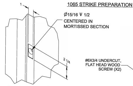
1. MARK AND MORTISE STRIKE ON JAMB TO MATCH LOCK POSITION ON DOOR - MORTISE 3/64" DEEP. DRILL Ø15/16" HOLE 1/2" DEEP IN CENTER OF MORTISE.
