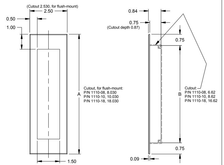
SUPPLIED WITH FOUR (4) #6 X 3/4" FLUSH HEAD SHEET METAL SCREWS
