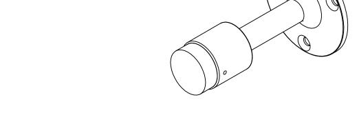
SUPPLIED WITH THREE (3) #8 X 1-1/4" OVAL HEAD, PHILLIPS DRIVE WOOD MOUNTING SCREWS.
