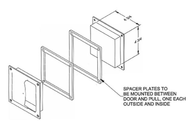
SUPPLIED WITH: FOUR (4) #8-32 X LENGTH FLAT HEAD, PHILLIPS DRIVE SEX BOLTS THE LENGTH OF WHICH IS DETERMINED BY THE DOOR THICKNESS, STANDARD IS 1-3/4"
