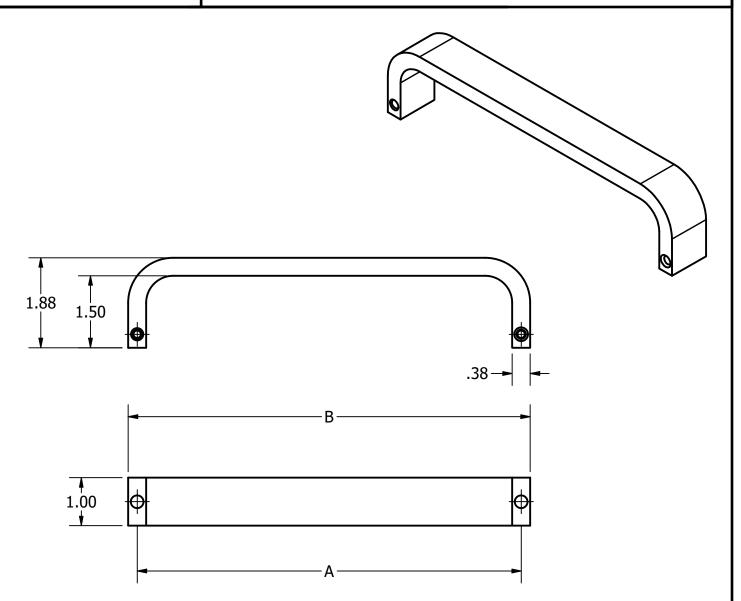
SUPPLIED WITH TWO (2) 1/4-20 SHOULDER BOLTS AND FOUR (4) 10-32 SET SCREWS. FOR WOOD DOORS, (2) BUSHINGS FOR HOLLOW METAL DOORS, (2) RIV-NUTS
