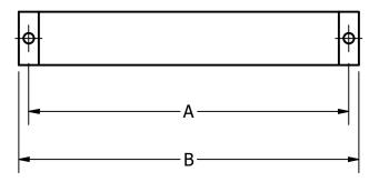
SUPPLIED WITH TWO (2) 1/4-20 FLAT HEAD, PHILIPS DRIVE MACHINE SCREWS AND TWO (2) 1/4 FINISH WASHERS.
